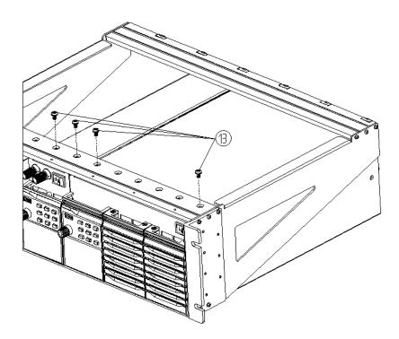
5. Secure the blank panels with the PM3×6 screws 1 and KM3×6 screws 12.
